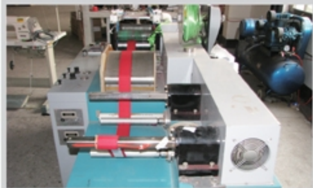
Ribbon Edge Embossing Machine (Ultrasonic) 分条缎带压边机
